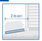
2 Extend downspouts and sump discharge pipes at least 2 m from foundation.
